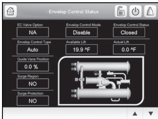
Fig. 38 — Envelop Control /HGBP (Hot Gas Bypass) Status
